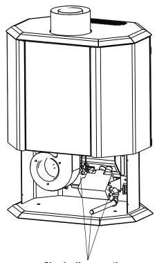
Check all connections for leaks using a gas Figure 28 leak test solution.
